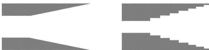
Fig. 6. A conventional smooth conical horn (left) and the proposed conical horn with hard surfaces (right)
