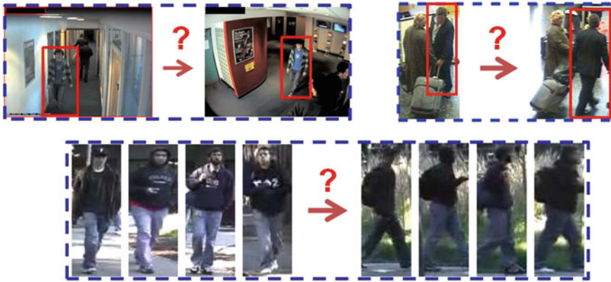
Fig. 20.1 An illustration of the difficulties of visual matching across different camera views. Individuals may undergo significant variability in appearance due to changes in lighting, scale and viewpoint. Other difficulties are caused by partial or complete occlusion which results in a lack of complete visual information, and the tendency for variability between people (inter-variation) to be less than the variability for a single person at different times and camera views (intra-variation). All of these problems are compounded by spatially large environments with significant numbers of cameras and levels of crowding
