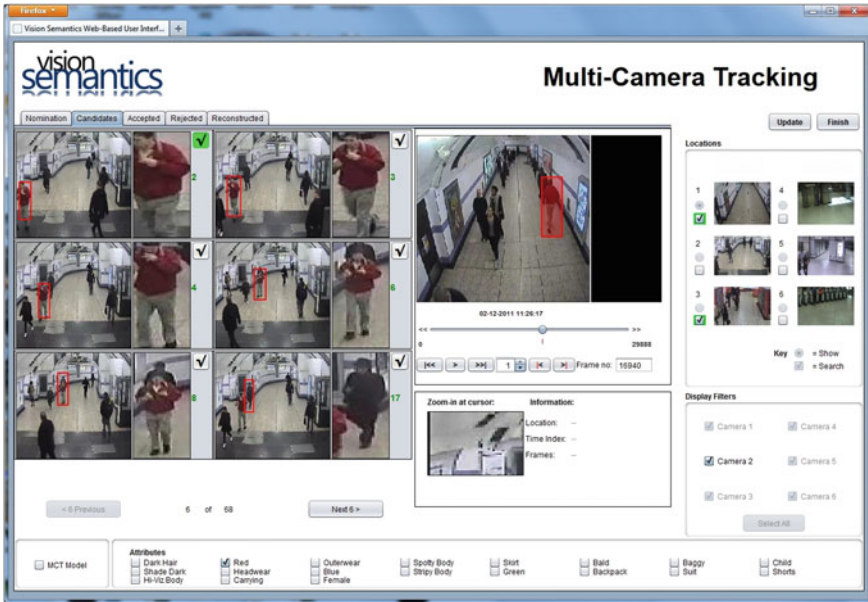
Fig. 20.5 MCT User Interface Client example screenshot. Here, users examine a paginated set of match candidates from a search iteration, locating and tagging those relevant including target associates. The local space–time profile Convergent Querying filter is employed here, using tagged candidates to immediately narrow the set being displayed to the appropriate temporal window. Attributes appropriate to the target may also be selected, which instantly re-rank the candidate list accordingly
