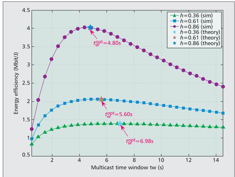
Figure 6. Performance of the proposed scheme: energy efficiency vs. time window ( $t_w$ ) under various user behaviors  $h$ .
