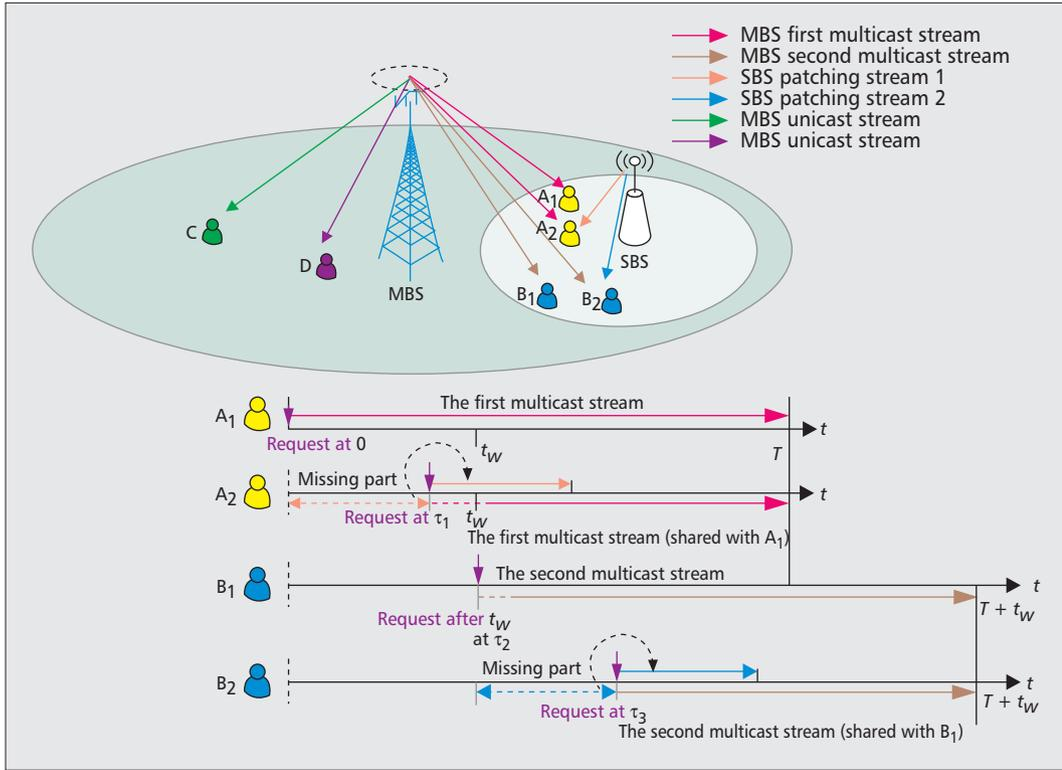
**Figure 4.** Detailed illustration of the proposed paradigm for energy-efficient multimedia transmission through base station cooperation.
