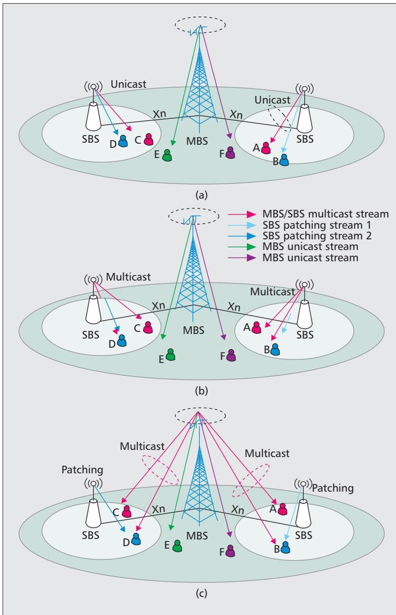
**Figure 3.** Illustration of multimedia service transmission in heterogeneous cellular networks: a) unicast multimedia transmission; b) traditional multicast multimedia transmission; c) proposed paradigm for multimedia transmissions through base station cooperation exploiting user behavior.
