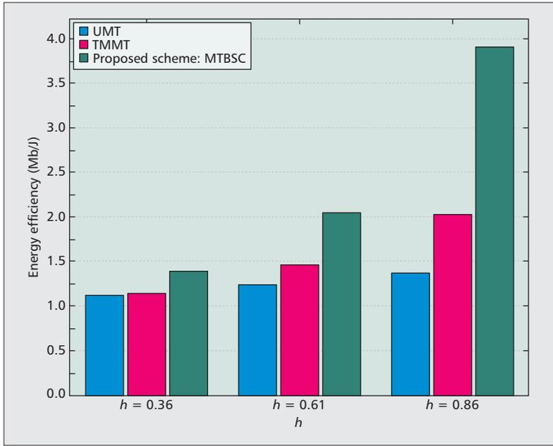
**Figure 5.** Energy efficiency vs. user behavior coefficient  $h$  for three multimedia transmission schemes in HCNs.
