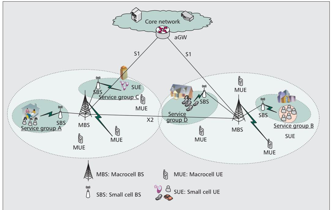
Figure 1. Architecture of heterogeneous cellular networks.
