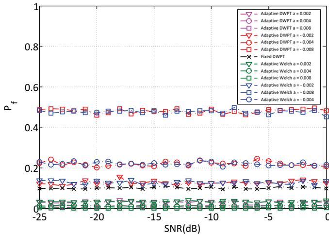
Fig. 5:  $P_f$  versus SNR for fixed/adaptive DWPT and Welch algorithms with different influence ratio  $\alpha$
