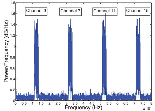
Fig. 3: A graphical illustration of the PSD for 16 LTE channels where channel 3,7,11 and 15 are occupied (SNR=10dB).
