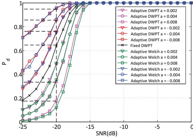
Fig. 4:  $P_d$  versus SNR for fixed/adaptive DWPT and Welch algorithms with different influence ratio  $\alpha$
