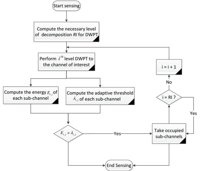
Fig. 1: A graphical structure of the flow Chart for adaptive DWPT based energy detection
