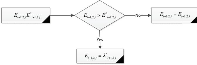
Fig. 2: A graphical structure of the energy component computation process for proposed adaptive threshold algorithm
