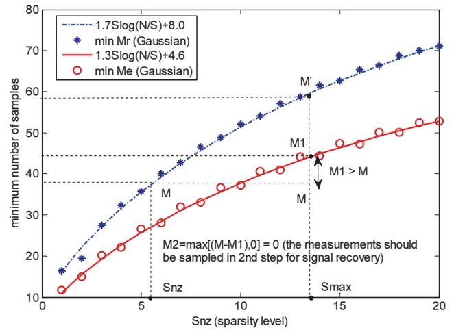
Fig. 2: Problem occurs when  $S_{nz}$  is too small compared with  $S_{\max}$ .
