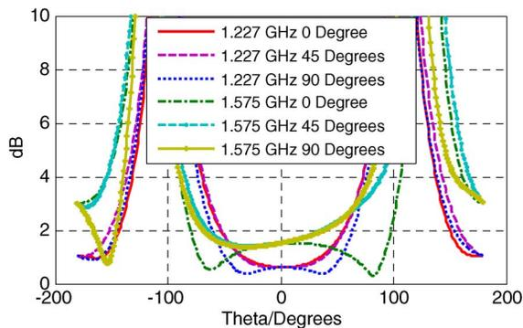
Fig. 9. Cartesian plot of the axial ratio of the proposed antenna at the boresight for 1.227 and 1.575 GHz at  $\phi = 0^\circ, 45^\circ, \text{ and } 90^\circ$ .
