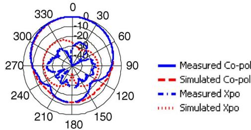
Fig. 8. Linear polarized radiation pattern at 1.8 GHz showing both the measured and simulated co- and cross polarization at  $xz$ -plane.
