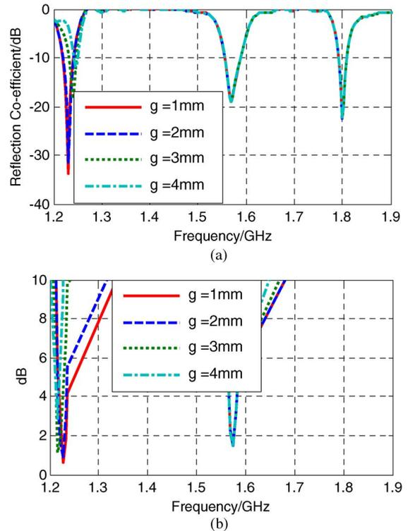
Fig. 2. Variation of the antenna parameters for different values of breadth  $g$  of I-slot in the lower patch: (a) reflection coefficient and (b) axial ratio.
