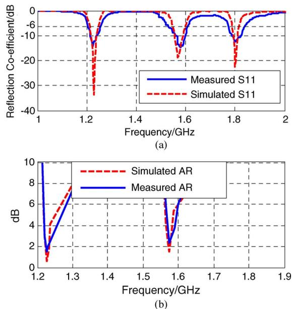
Fig. 5. Measured and simulated reflection coefficient and axial ratio of the proposed antenna: (a) measured and simulated reflection coefficient and (b) measured and simulated axial ratio.
