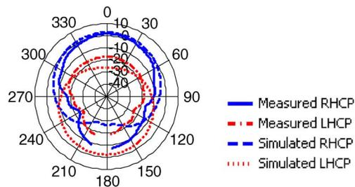
Fig. 6. Measured and simulated RHCP and LHCP radiation patterns in  $xz$ -plane of the proposed antenna at 1.227 GHz.
