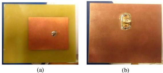
Fig. 4. Fabricated prototyped stacked-patch, triple-band, dual-polarized antenna: (a) top view and (b) bottom view.
