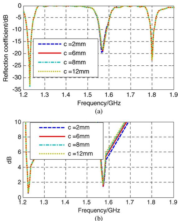
Fig. 3. Variation of the antenna parameters for different values of length  $c$  (middle patch I-slot): (a) reflection coefficient and (b) axial ratio.
