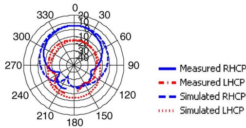
Fig. 7. Measured and simulated RHCP and LHCP radiation patterns in  $xz$ -plane of the proposed antenna at 1.575 GHz.
