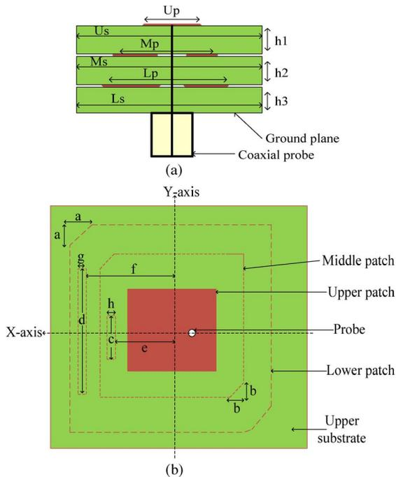
Fig. 1. Geometry of the proposed stacked-patch, triple-band, dual-polarized antenna. (a) Configuration of the antenna. (b) Top view of the antenna.
