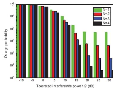
Figure 3. Outage probability vs. tolerated interference power.
