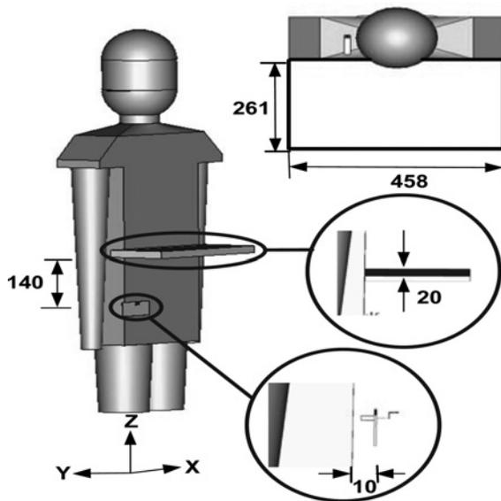
**Figure 14** On-body test configuration with horizontal handset and horizontal barrier (all lengths are in mm)
