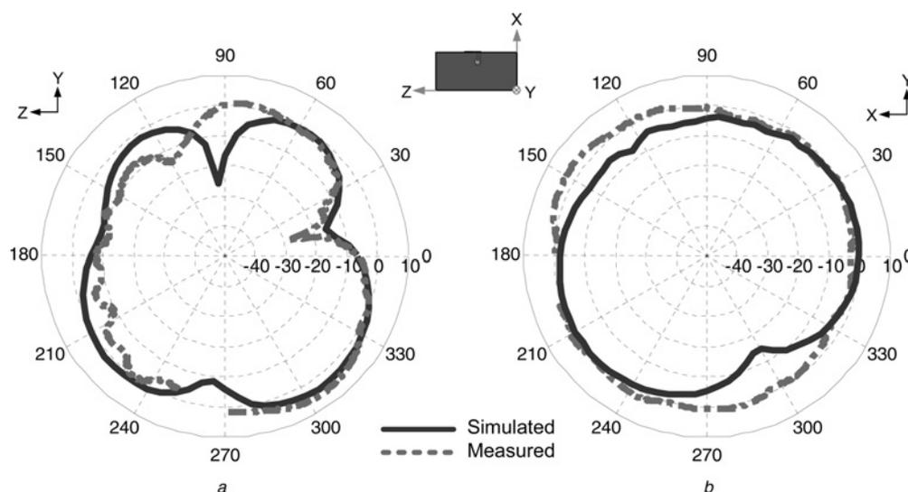
**Figure 4** Comparison of simulated (dark grey) and measured (light grey) 2-D radiation patterns of the PIFA handset antenna at 2440 MHz
