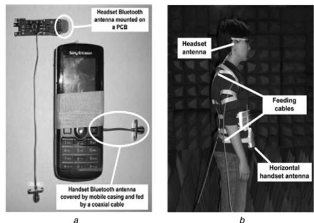
**Figure 7** Antenna prototypes and on-body test set-up used for the measurements
