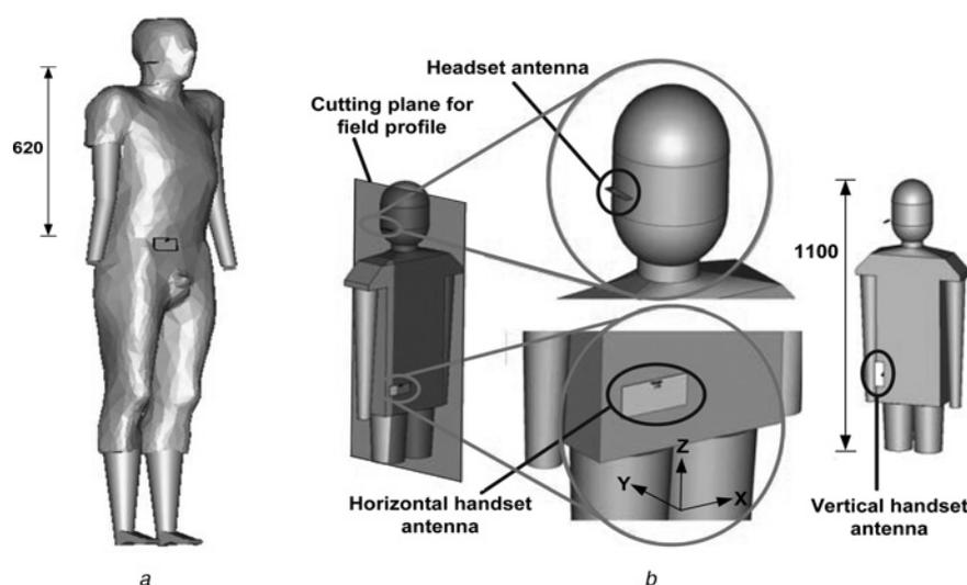
**Figure 5** Numerical models of the human body and on-body test configurations
