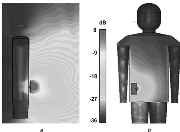
**Figure 10** Normalised electric field distribution and on-body surface waves for vertically oriented handset
