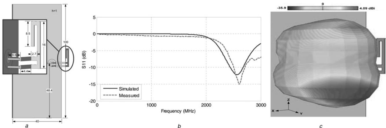
**Figure 3** Handset PIFA antenna geometry and performance for the Bluetooth operation
