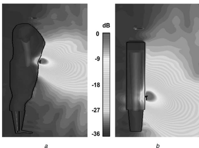
**Figure 6** Comparison of normalised electric field distributions and on-body surface waves on realistic body model and simple body model for horizontally oriented handset
