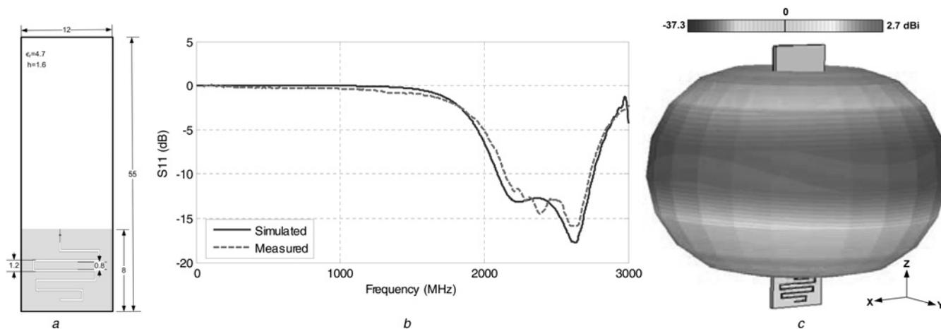
**Figure 1** Headset meander line monopole antenna geometry and performance for the Bluetooth operation
