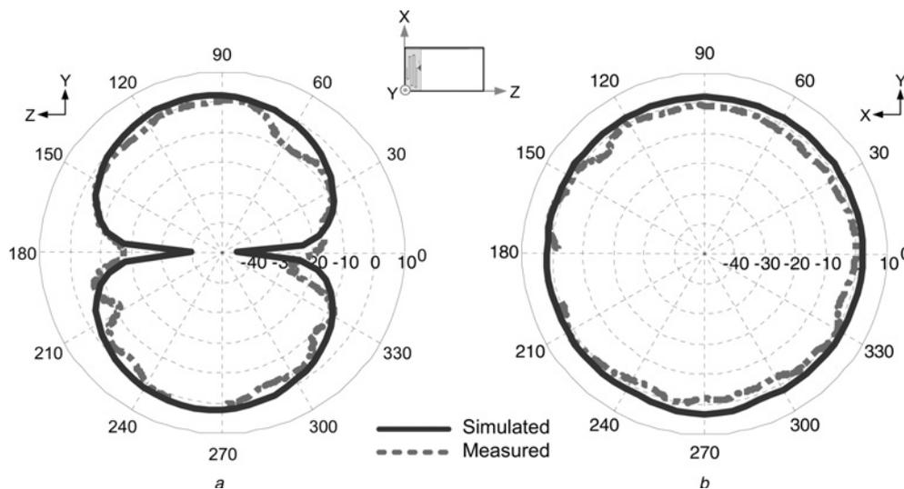
**Figure 2** Comparison of simulated (blue) and measured (red) 2-D radiation patterns of the Bluetooth headset antenna at 2440 MHz
