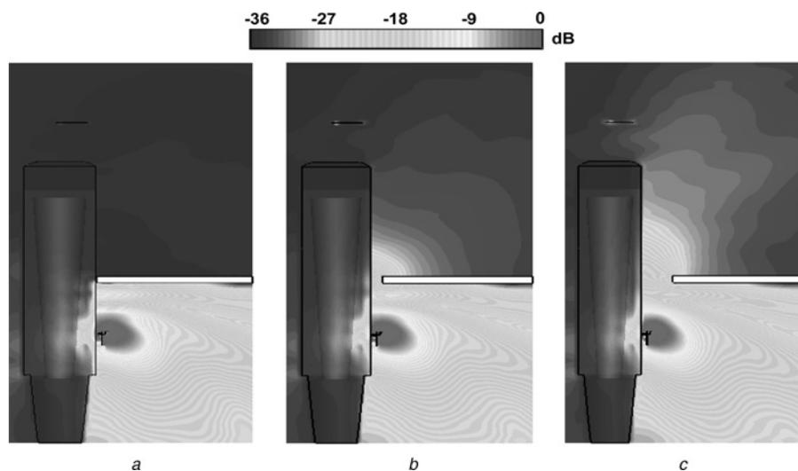
**Figure 15** Normalised electric field distribution and on-body surface waves for horizontal handset observed on the cross-section plane with barrier at different separations ( $d$ ) from the body surface
