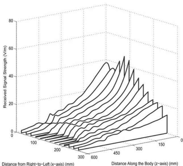
**Figure 12** Received signal strength on the path along the body surface between the vertical handset and the headset antennas, corresponding to Fig. 10b
