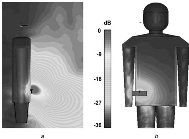
**Figure 9** Normalised electric field distribution and on-body surface waves for horizontally oriented handset
