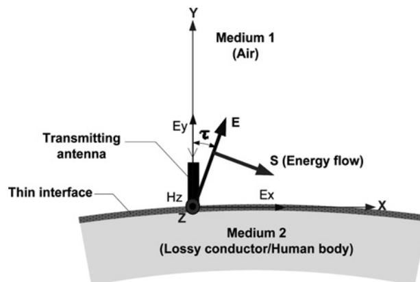
**Figure 8** Generation of surface waves on the interface of air and lossy conductor because of downward tilt of the wave-front
