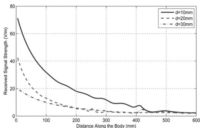
**Figure 13** Received signal strength along the body surface for different separations of horizontal handset and body
