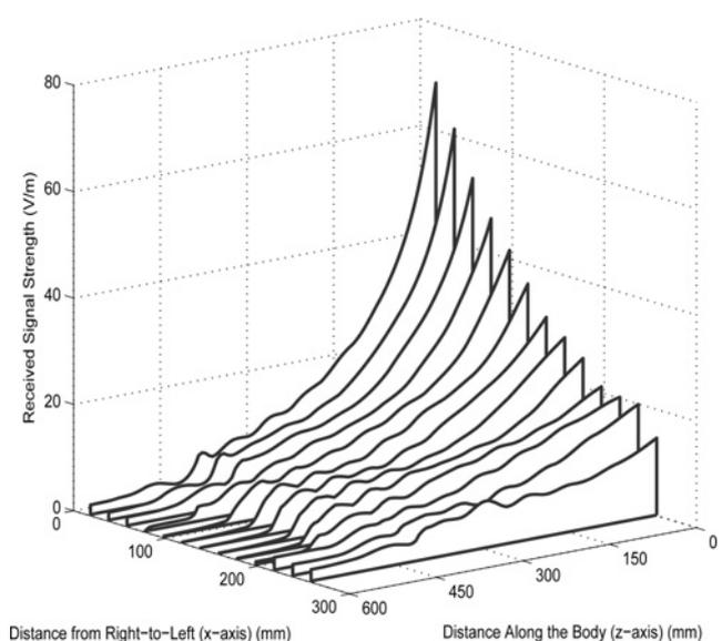
**Figure 11** Received signal strength on the path along the body surface between the horizontal handset and the headset antennas, corresponding to Fig. 9*b*
