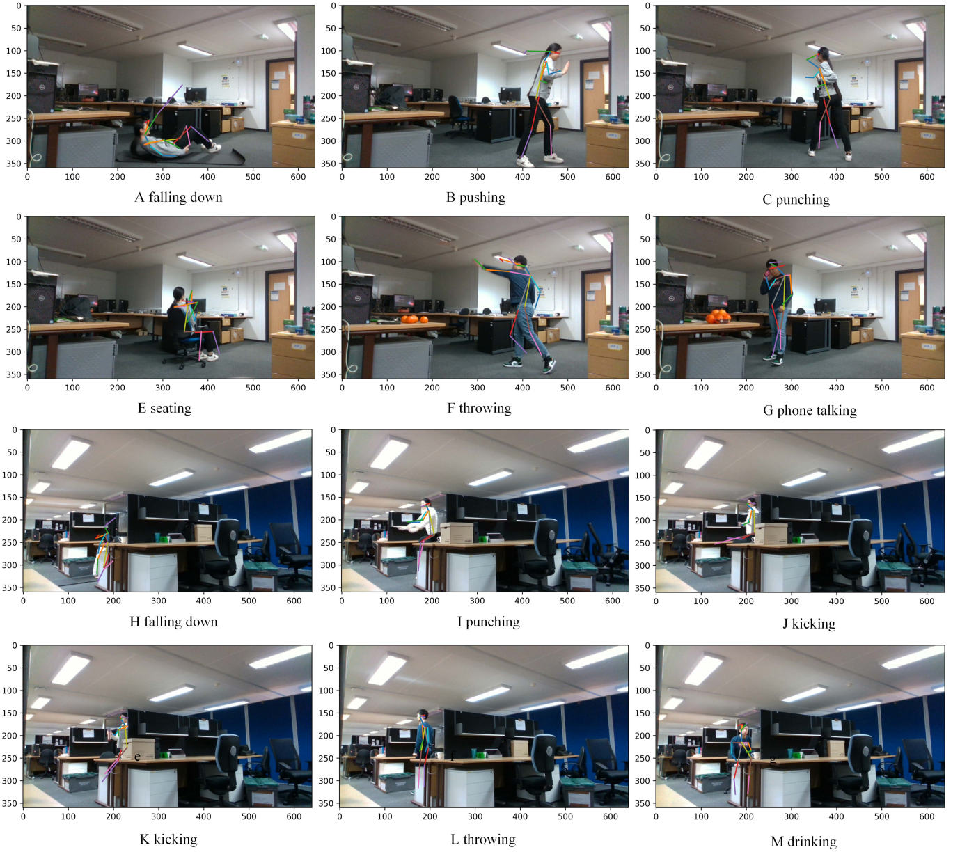
Fig. 9. The visual skeleton result of the CSI in two scenarios, where A-G are without occlusion scene, and H-M are partial occlusion scene.
