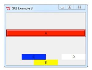
The desired behaviour is shown below. The four labels are positioned at the corners and the labels fill the space when the window is resized.
