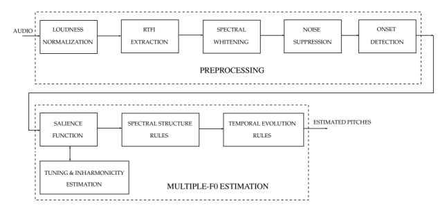
Figure 1: Diagram for the proposed multiple fundamental frequency estimation system.
