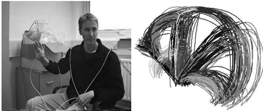
Figure 4: Experimental Setup: The Polhemus tracker with sensors attached to the right hand and head (left). The recorded input sequence segmented into 668 atomic components (right).
