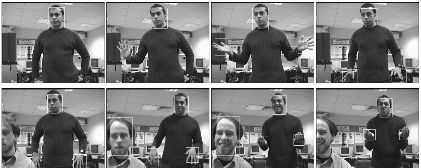
Figure 5. Focus of attention for face and gesture recognition using a multi-object colour tracker. The system runs at around 15Hz on a 200MHz PC.
