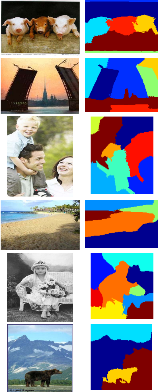
Figure 2: Examples of image segmentation. Left: original images; Right: segmentation results. From top to bottom, the optimal number of segments K_o were automatically determined as 7, 7, 8, 5, 9, and 4 respectively.
