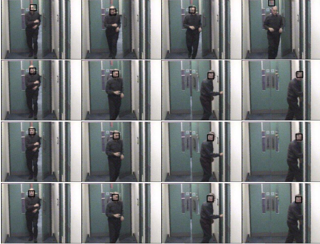
Figure 1. Experiments 1, 2, 3 and 4: The four rows of images represent four separate video sequences produced by four experiments respectively. In the first experiment (first row), only 5 random samples are picked from each of the candidate and model images, 10 samples in the second experiment (second row), 15 samples in the third (third row) and 150 samples in the fourth (fourth row).
