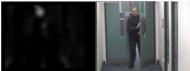
Figure 7. Object Detection using Color Distributions with the Number of Samples 10
