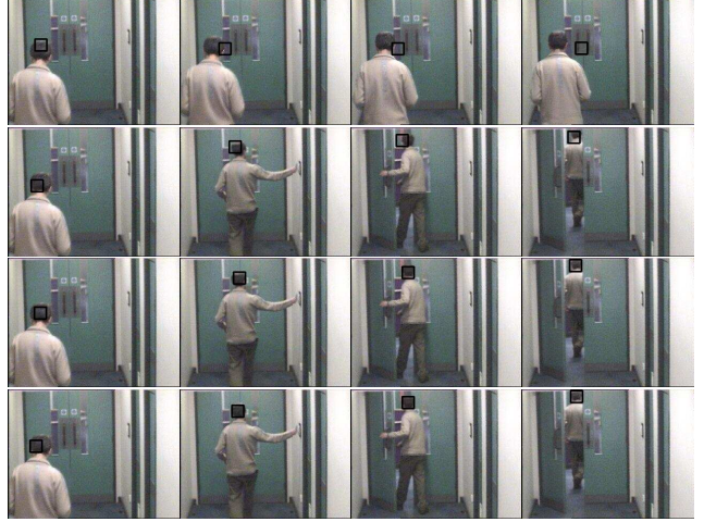
Figure 2. Experiments 5, 6, 7 and 8: The four rows of images represent four separate video sequences produced by four experiments respectively. In Experiment 5 (first row), only 2 random samples are picked from each of the candidate and model images, 3 samples in Experiment 6 (second row), 5 samples in Experiment 7 (third row) and all samples from the candidate and model images (traditional Mean-Shift tracking) in Experiment 8 (fourth row).
