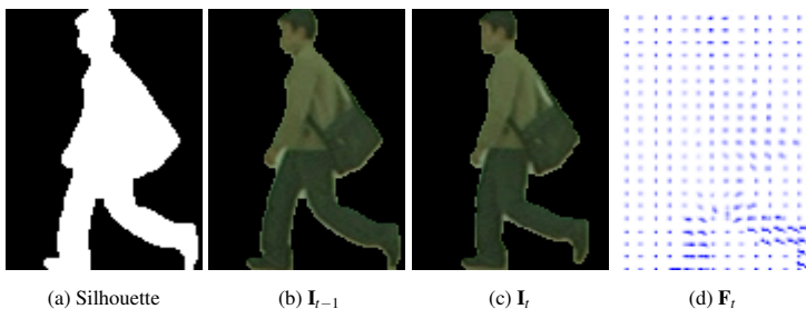
Figure 1: Computing figure-centric optical flow field. (a) shows the silhouette at frame t - 1 ; (b)&(c) are the extracted figure-centric images of the walking person at t - 1 and t respectively; (d) is the computed optical flow field.
