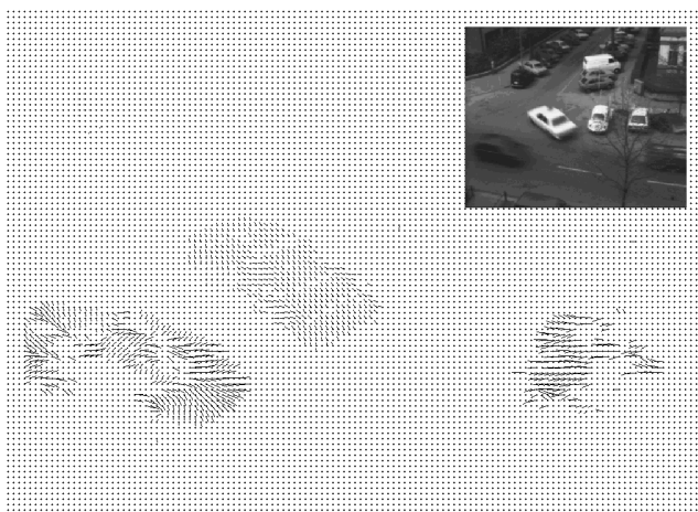
Figure 2 Recovered optical flow field for traffic sequence. The needle diagram illustrated shows the direction and speed of the motion at each point in the field. The length of the needle represents speed. A representative image from the traffic sequence used is shown inset at top right.
