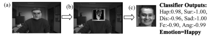
Fig. 1. System summary. (a) Face in the scene is located using a face tracker. (b) Motion of the face region only is determined using an optical flow algorithm. (c) Processed motion data is input into SVM classifiers. The motion signature is labeled as either one of the six basic emotions or as nonexpressive according to classifier outputs. In this case, the sequence is labeled as happiness as the highest output is happiness (0.98) and this value exceeds the required expression—nonexpression threshold.
