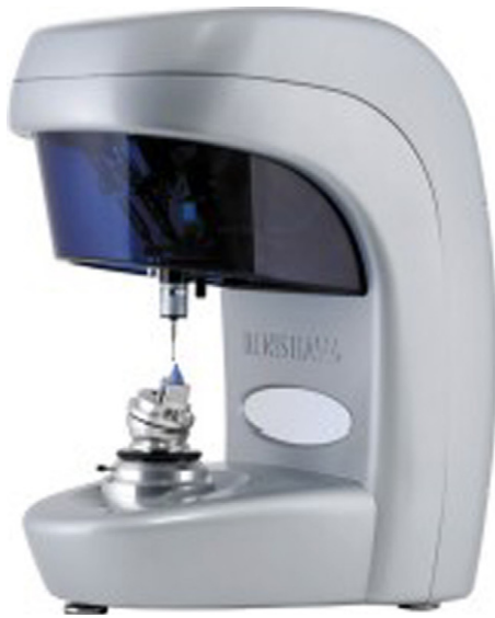
Fig. 1. Incise dental scanner (Renishaw, UK), (Courtesy of Renishaw PLC).
