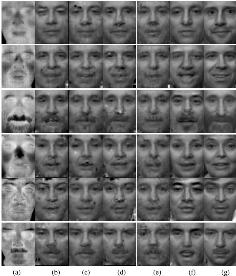
Fig. 2. The results of face image conversion from thermal infrared images. (a) the input infrared image; (b) the result of our method using the prediction method of LLR using 5 canonical variates for each patch; (c) the result of our method using the prediction method of Sophisticated LLE; (d) the reconstruction face using 5 canonical features for each patch extracted from the ground truth; (e) the result using directly LLE method; (f) the result using the holistic method; (g) the ground truth.
