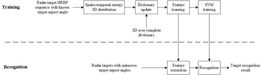
Fig. 2. The model of the proposed moving target recognition system.
