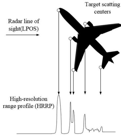
Fig. 1. An example of a plane target HRRP sample and scatters. This picture is cited from [9].
