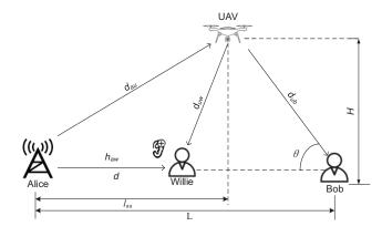
Fig. 1. Covert communication from Alice to Bob assisted by a UAV relay under the detection of Willie
