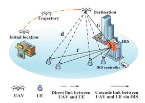
Fig. 1. IRS empowered UAV downlink communications network.
