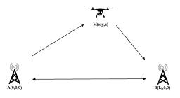
Fig. 1. A rotary-wing UAV relay in a three-node communication system.
