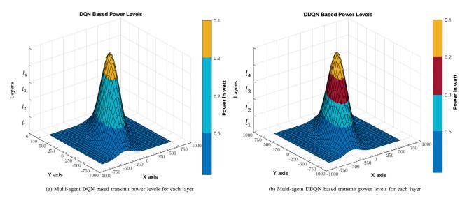
Fig. 9: Multi-agent DQN based transmit power levels vs. Multi-agent DDQN based transmit power levels for each layer: In Sub-figure (a) IoT users in layer 2 and 3 use same power level, whereas, in Sub-figure (b) IoT users in different layers select different transmit power levels for GF transmission that ensure sufficient received power difference at the BS.
