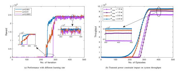
Fig. 6: The learning rate comparison and impact of transmit power constraint: Sub-figure (a) represents the performance comparison with different learning rates. Sub-figure (b) shows the impact of transmit power constraint on the system throughput.
