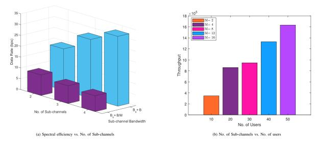
Fig. 7: Spectral efficiency versus the number of sub-channels M: Sub-figure (a) shows two cases: First, The system bandwidth B is equally divided into M orthogonal sub-channels and thus each sub-channel has  $B_s = \frac{B}{M}$  available bandwidth and secondly, bandwidth of each sub-channel  $B_s = B$ . Sub-figure (b) represents system throughput w.r.t, increasing number of users and sub-channels.
