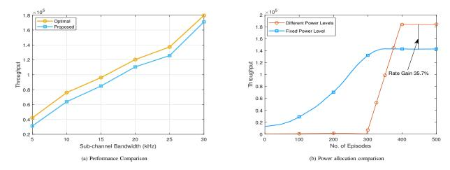
Fig. 8: Performance and power allocation comparison with M=4 and  $N_t=6$  (active users): Sub-figure (a) shows system performance with varying sub-channel bandwidth as compared to optimal solution. Sub-figure (b) represents the performance comparison in terms of throughput achieved by allocating fixed power to IoT users and power allocating from the available power pool.
