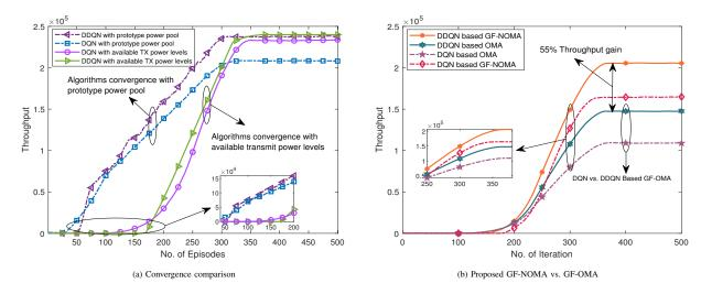
Fig. 10: Convergence comparison and performance of the proposed GF-NOMA vs. GF-OMA: Sub-figure (a) shows Comparison of the proposed multi-agent DRL based GF-NOMA algorithms (multi-agent DQN based GF-NOMA and multi-agent DDQN based GF-NOMA) with and without the prototype power pool. Sub-figure (b) represents the comparison of proposed multi-agent DRL based GF-NOMA and GF-OMA.
