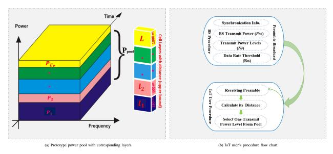
Fig. 2: The designed prototype power pool and working procedure of the BS and IoT users: Sub-figure (a) is the transmit power pool with different power levels for each layer. Sub-figure (b) shows the procedure flow chart between the BS and IoT users.
