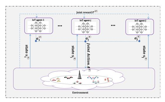
Fig. 3: The MARL framework for GF-IoT Networks, where IoT agents takes joint actions and receives a common reward during the training process to learn the optimal policy.
