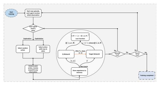
Fig. 4: The proposed end-to-end architecture for training deep MARL agents to optimize the power and sub-channel allocation.
