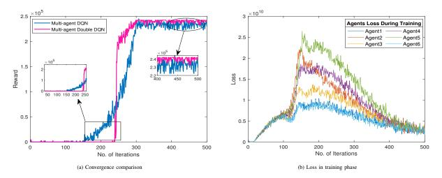
Fig. 5: The convergence of multi-agent DRL based GF-NOMA algorithms and the loss in the training phase: Sub-figure (a) shows the convergence of the proposed multi-agent DQN based GF-NOMA vs. multi-agent double DQN based GF-NOMA algorithm. Sub-figure (b) represents loss function value of all agents ( $N_t = 6$ ) in the training phase. At each time step, the stochastic gradient descent algorithm minimizes the loss function mentioned in (23) for training the mini-batch.
