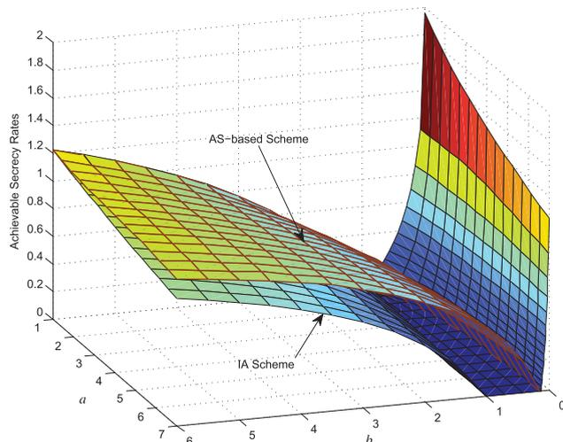
**FIGURE 2.** Achievable secrecy rates of the IA and AS-based schemes for the WT-HI channel shown in Fig. 1 (a), where the maximum transmit power at Alice and Carlo are 20 and 50, respectively. Since the IA scheme is a generalization of the CJ and NF scheme, its achievable secrecy rate is the same as that of the CJ scheme when  $b < 1$  and the same as that of the NF scheme when  $b > 1$ .
