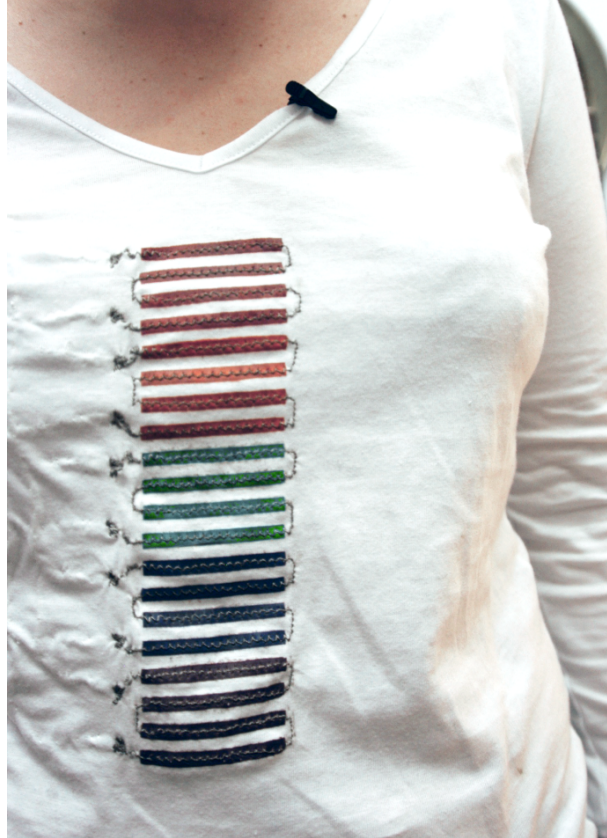
Fig. 3. The display is constructed with heat-sensitive paints and conductive thread in the shape of a bar chart. The higher the compatibility level, the more heat is provided to the display causing the bar chart, initially black, to become more colourful
