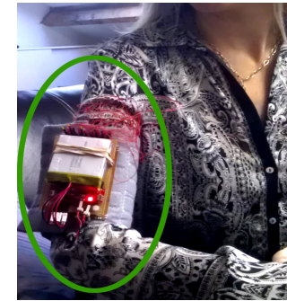
figure 7. A test subject wearing Vibrosign with a controller circuit, battery pack and motor circuit attached on the outer side of the armband.
