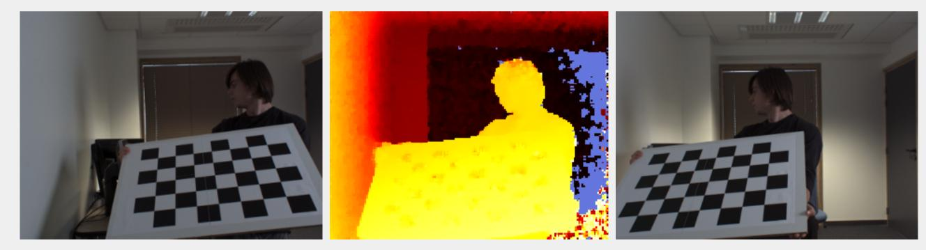
▶ Reprojection of the 3D range-points, via new cameras  $C'_{l}$  and  $C'_{R}$ :
