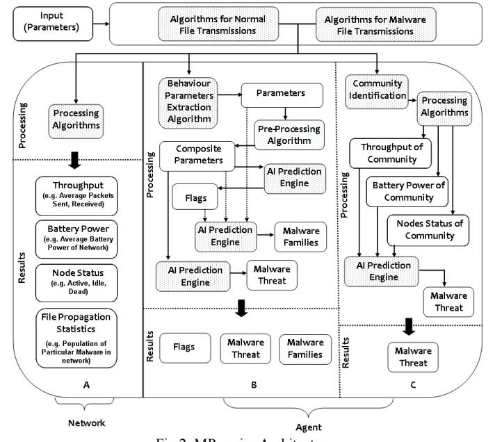
Fig.2. MPeersim Architecture
