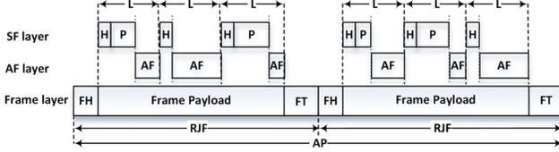
Fig. 3: The layered structure of Flexilink
