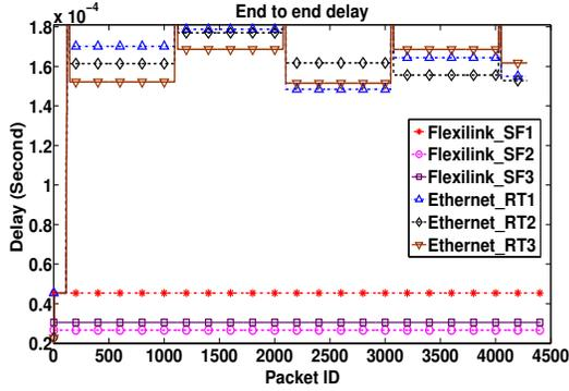
Fig. 8: Detailed E2E delay for SF in Case Three
