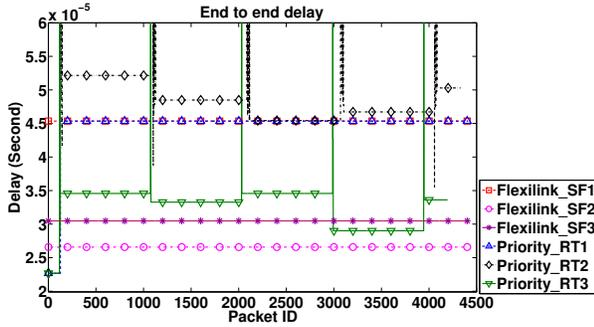
Fig. 11: Detailed E2E delay for SF in Case Four
