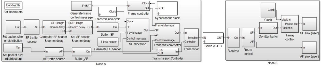
Fig. 4: The Flexilink network architecture
