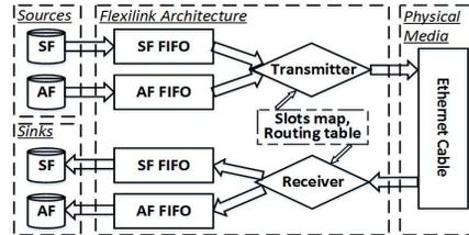
Fig. 2: The MAC layer design of Flexilink
