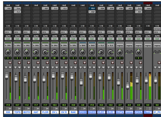
Figure 1. The fader view of a mix in ProTools, a typical mixing interface.
