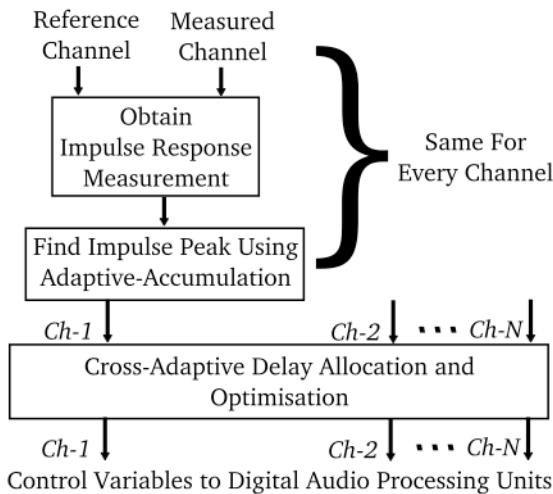
Figure 4 General algorithm flow diagram for an automatic mixture cross-adaptive time offset corrector.
