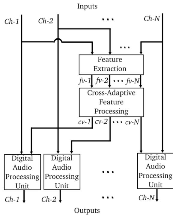
Figure 3 General cross-adaptive effect diagram.  $ch-1$  to  $ch-N$  are audio signals,  $fv-1$  to  $fv-N$  are the features extracted from the audio channels and  $cv-1$  to  $cv-N$  are the control vectors that drive the digital audio processors.
