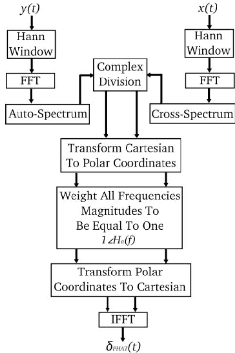
Figure 5 Robust impulse response measurement flow diagram, implemented using the PHAT method.
