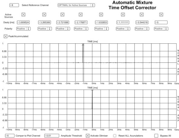
Figure 8 Master User interface of the implemented cross-adaptive time offset corrector.
