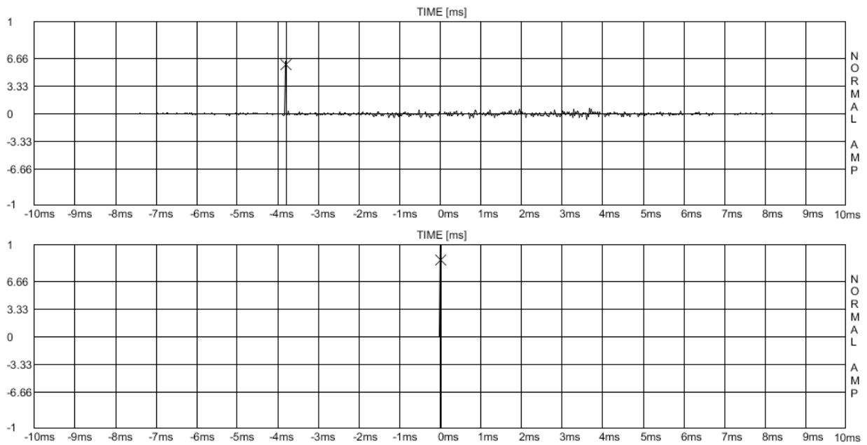
Figure 11 Measurements of impulse response of signal before correction (top) and after the correction (bottom). Measurements were made for a highly correlated signal.
