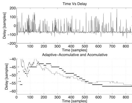
Figure 6 Non-accumulated  $\Delta(t)$ , (top). Comparison of accumulated  $\Delta_a(t)$  in gray, vs. accumulative adaptive validation  $\Delta_{am}(t)$  in black, (Bottom)
