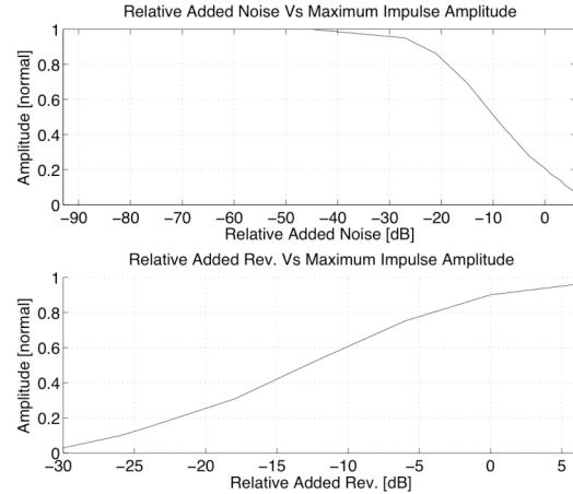
Figure 9 Impulse Response amplitude change due to the addition of noise (top). Impulse Response amplitude change due to the addition of reverberation (bottom). Measurements were performed for an impulse with no delay between reference and measured signal for a 0 sample error. The reverberation and noise were added to the measurement channel only.
