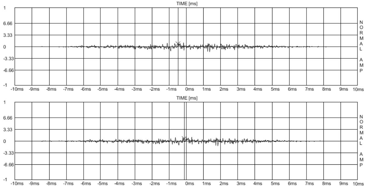
Figure 12 Measurements of impulse response of signal before correction (top) and after the correction (bottom). Measurements were made for a low correlated signal.
