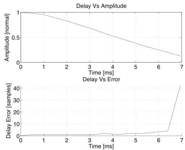
Figure 10 Impulse response amplitude windowing effect as a function of the delay offset between the reference channel and the measured channel (top). Delay calculation error as a function of the delay offset between the reference channel and the measured channel (bottom).
