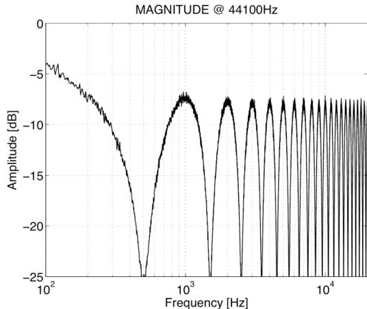
Figure 1 Comb Filtering of two white noise signals, both having the same amplitude, with a, 1ms delay between them.
