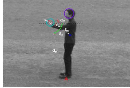
Figure 1. An overview of the stored spatial parameters per each codeword pair during the learning phase. For illustration purposes, only the position parameters for one of the constituent codewords are depicted.
