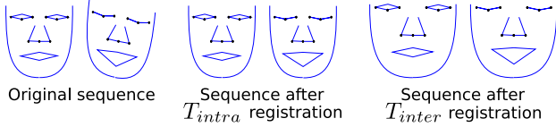
Fig. 3: An illustration of the rigid registration process. Also shown are the 10 facial feature points used for registration.
