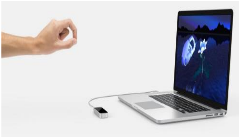
Figure 11: The LM Usage. The hand above the LM interacts with virtual objects [53].
