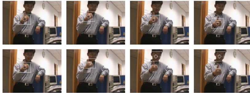
Fig. 12. Comparison between two different observation models for one test sequence (frames 5 to 8). Top row: Observation model based on color and motion cues. Bottom row: Observation model based on color cue only. The video demo V1 is available online.
