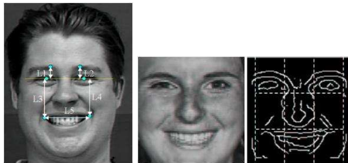
Fig. 8 Geometric features (Tian, Brown, Hampapur, Pankanti, Senior, and Bolle, 2003): (Left) location features; (Right) normalized face and zones of the edge map of the normalized face.
