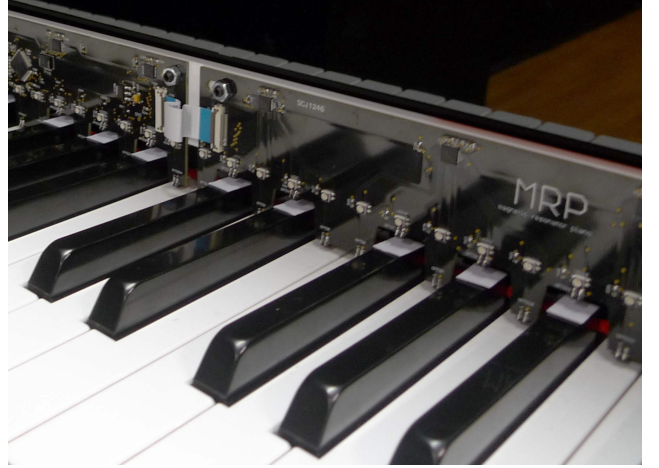
Figure 1: Optical scanner hardware. Top: scanner showing all RGB LEDs active, set up on the magnetic resonator piano. Bottom: optical sensors over each key. White stickers are attached to the black keys to increase their reflectance.
