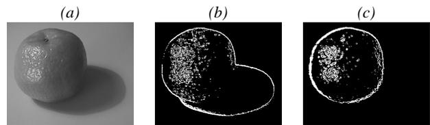
**Fig. 1.** Edge detection on luminance and photometric invariant: (a) original image; (b) edge map of the luminance component containing object and shadow boundaries; (c) color edge map on invariant color features containing only the object boundaries.
