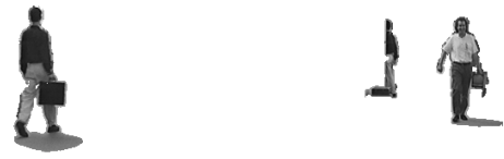
Figure 2: Examples of change detection results. Objects as well as their shadows are segmented
