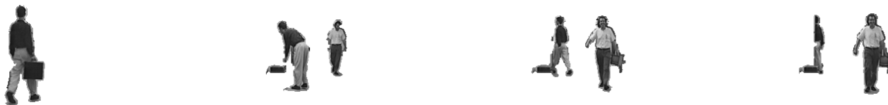
Fig. 11. Semantic video object extraction results for sample frames of the test sequence Hall Monitor
