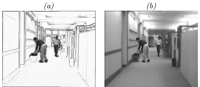
Fig. 14. Example of use of the proposed semantic video object extraction algorithm. (a) The extraction of moving objects allows one to reconstruct a scene with a simplified background, thus enhancing the visibility of the moving objects. (b) Example of use of semantic video object extraction for preprocessed frame before coding: the background information is blurred thus requiring less bandwidth while still retaining essential contextual information
