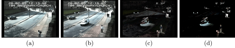
Fig. 1. Contrast enhancement for improving object detection. (a) Reference frame; (b) current frame; (c) image difference before contrast enhancement; (d) image difference after contrast enhancement.
