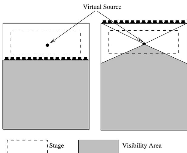
Figure 1: WFS setups for creation of "on stage" virtual source
