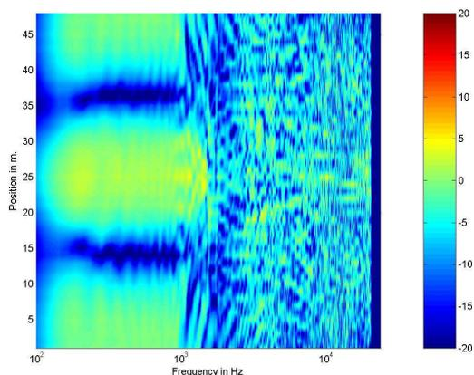
Figure 4: Frequency responses of a 5th order cylindrical harmonics
