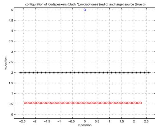
Figure 2: MAP reproduction setup. Crosses correspond to the loudspeaker positions, red circles to the microphones and the blue circle to the target source
