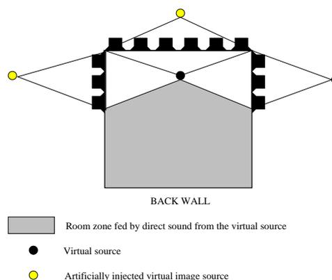
Figure 5: Artificial injection of virtual image sources using loudspeaker arrays along front and side walls of the listening room.
