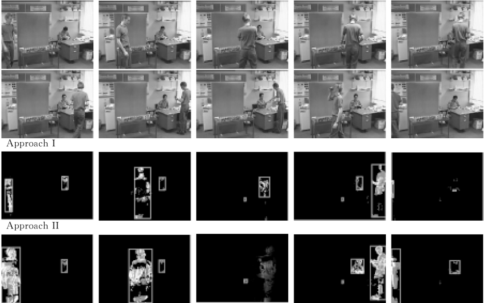
Fig. 1 Autonomous event detection in a simulated shopping scenario. The figures in the top two rows from left to right, top to bottom are the typical scenes of the shopping scenario, which were sampled from frame 110 to frame 330 of the 20 minutes video. The figures in the third and the fourth rows are a number of autonomous events detected using Approach I and Approach II respectively. Pixel-level events that satisfied Condition (3) in Section 2.2 were highlighted in white and those that did not were in grey. Recognised blob-level scene events were indicated with bounding boxes
