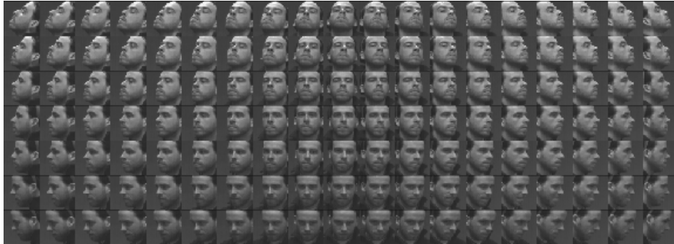
Figure 2: An example labelled head image set. The images of labelled views are from +90^\circ to -90^\circ in yaw and from +30^\circ to -30^\circ in tilt at 10^\circ intervals.
