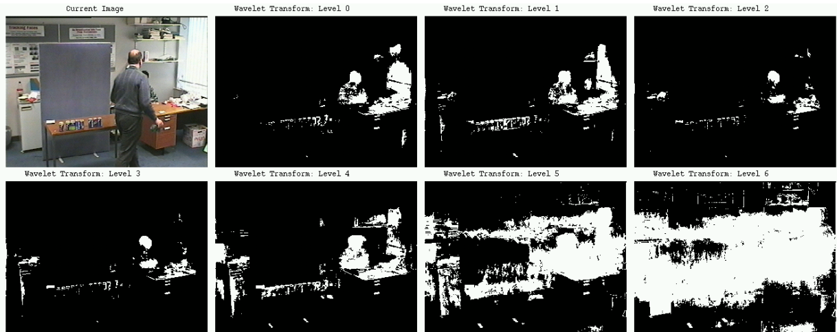
Figure 7. 7 level wavelet histogram of the shop scenario. From left to right, top to bottom, the figures are: original scene, then thresholded histograms in binary form from level 7 to level 1.
