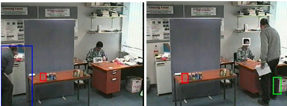
Figure 6. Example event detections. Blue box indicates browsing. Red box indicates can taken. White box indicates shop-keeper moving. Green box indicates paying.
