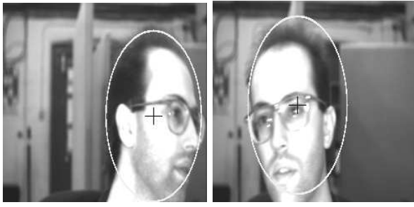
Fig. 6: Face detection and segmentation on a camera input sequence.
