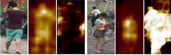
Figure 3. Illustration of the interference to the ReID objective when the weak saliency label is inaccurate. Each sample is presented with three columns: the input pedestrian image on the left, the activation from the primary ReID head in the middle, and the weak label for the auxiliary saliency detection head on the right. The gradient descent directions for the two objectives are contradictory.
