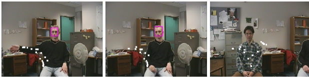
(b) System responding to pointing gesture by panning to other subject.
